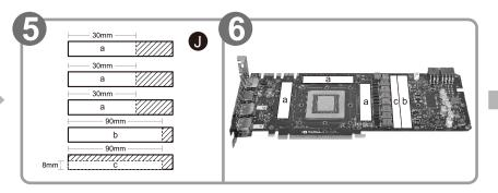
Cut the thermal pads to the dimensions listed and place them on the spots shown on the diagram.
