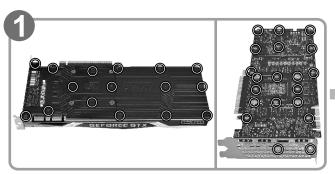
Remove original VGA stock cooler (Remove the screws circled on the diagram. All heat sink assembly screws should be removed)
